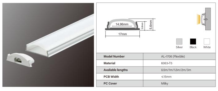
New Bendable Aluminum LED Profile (AL-1706 Flexible) is ideal for straight linear runs or it can bend and shape to surfaces that are non-linear making installation easier for curved shapes. Made from high quality Aviation 6063-T5 aircraft aluminum and Anodized, and can be used with LED Strip Light that are 8~12mm wide.
